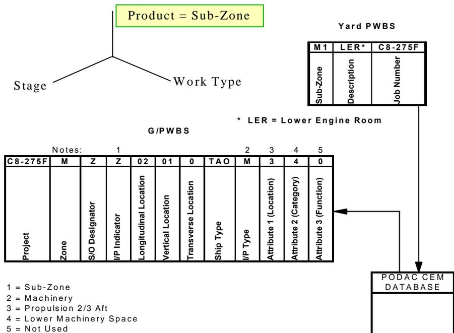
Figure 4. Mapping shipyard PWBS to G/PWBS, sub-zone.
