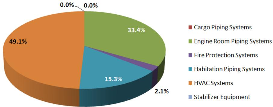
**100 meter 30 Kt Surface Combatant Auxiliary Systems - % Material & Equipment Cost Drivers**
