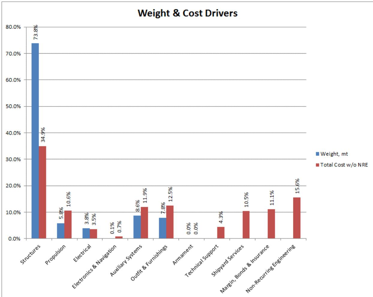
**Figure 5b: SPAR Cost Model Reported Weight & Cost Drivers for a Sample Ro-Ro Vessel**
