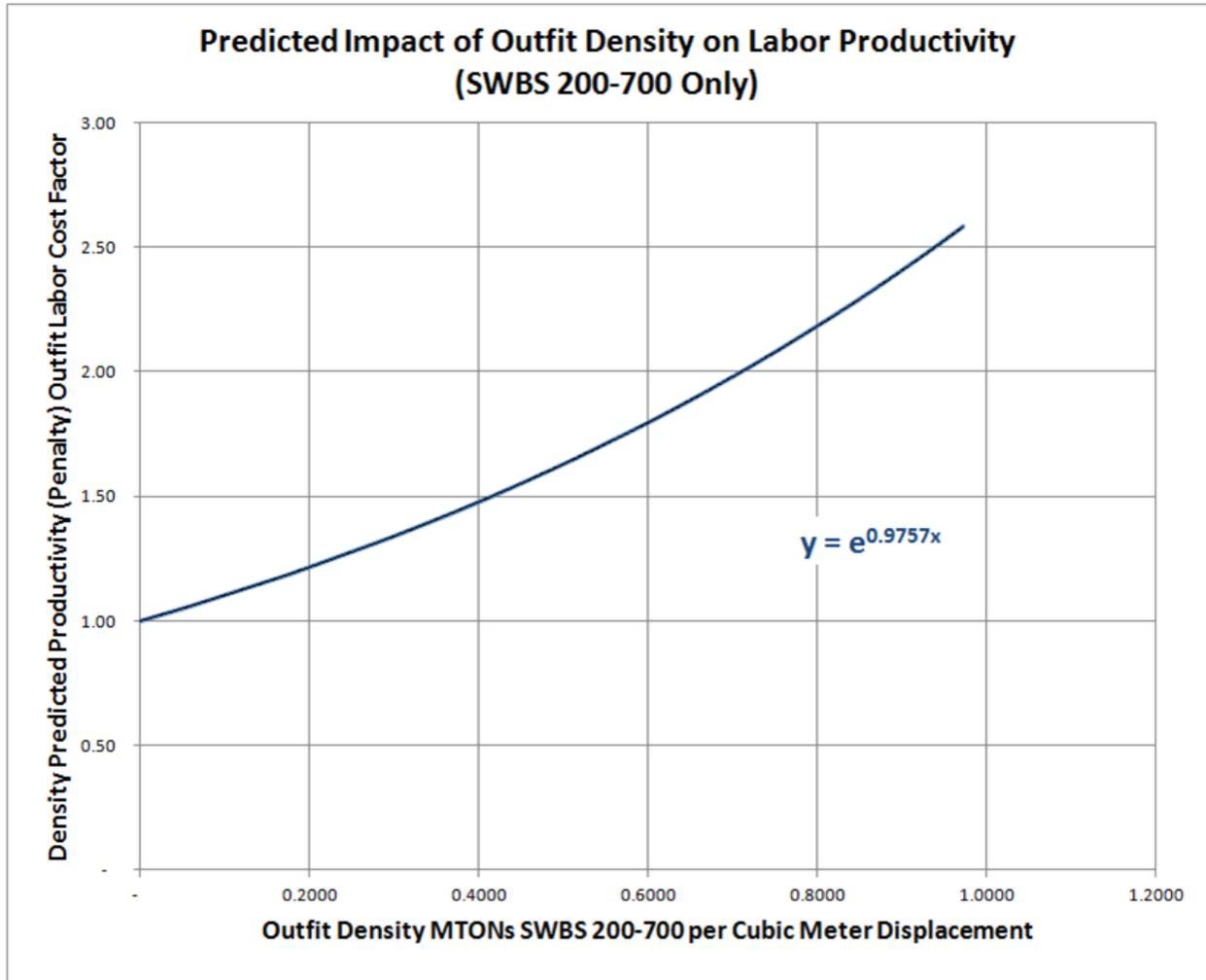
**Figure 10: Predicted Impact of Outfit Density on Labor Productivity.**
