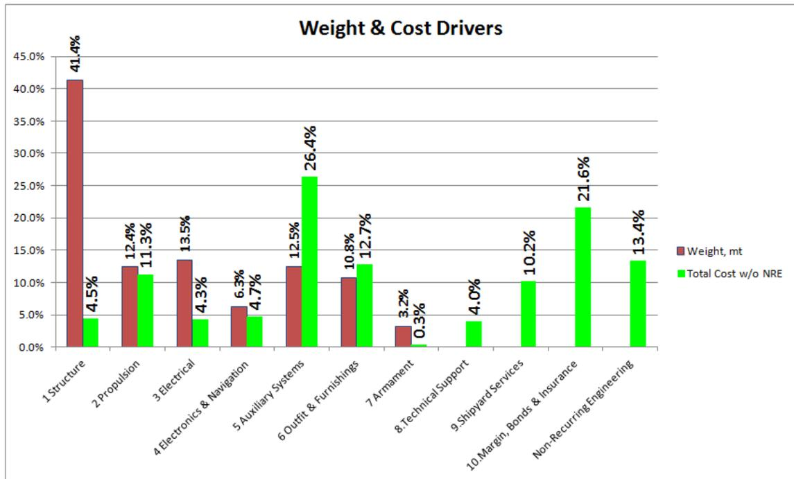
**Figure 5a: SPAR Cost Model Reported Weight & Cost Drivers for a Sample Patrol Vessel**
