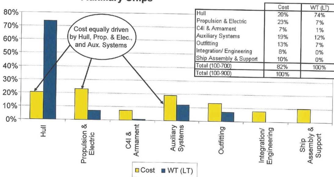
**Figure 4: NAVSEA Cost Drivers for Auxiliary Ships**
