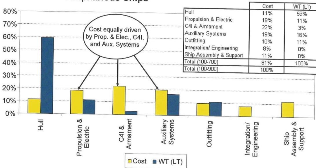
**Figure 3: NAVSEA Cost Drivers for Amphibious Ships**
