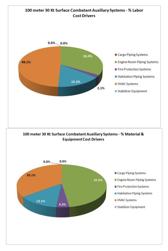
Figure 6: Summary of Labor Hours & Material Costs for Auxiliary Systems
