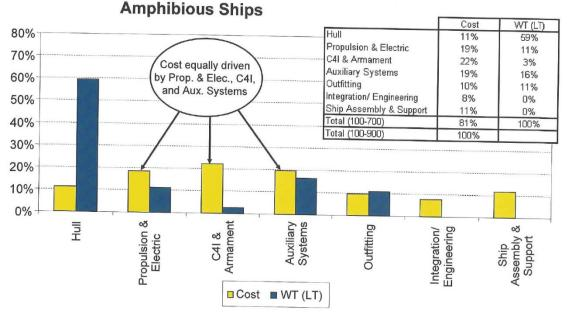
Figure 3: NAVSEA Cost Drivers for Amphibious Ships
