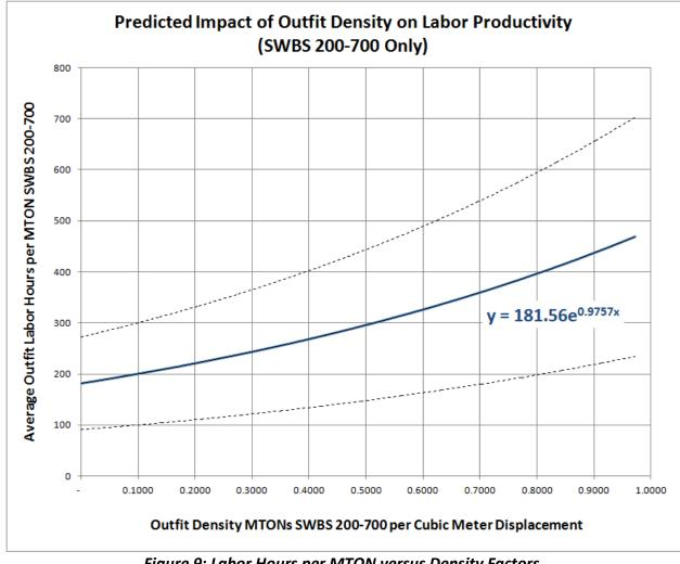
Figure 9: Labor Hours per MTON versus Density Factors
