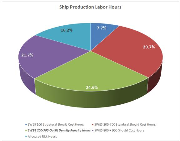
Figure 12: Breaking Out Standard Should Cost and Outfit Density Penalty Cost Labor Hours in Percentages
