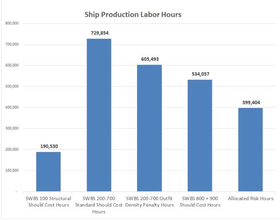
Figure 11: Breaking Out Standard Should Cost and Outfit Density Penalty Cost Labor Hours
