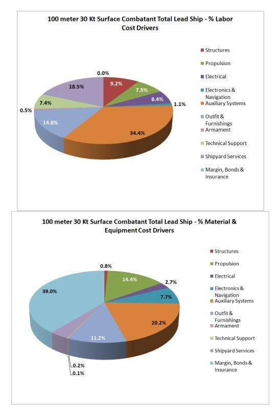
Figure 1: Average Percent Breakout of Production Labor Hours & Material/Equipment Costs
