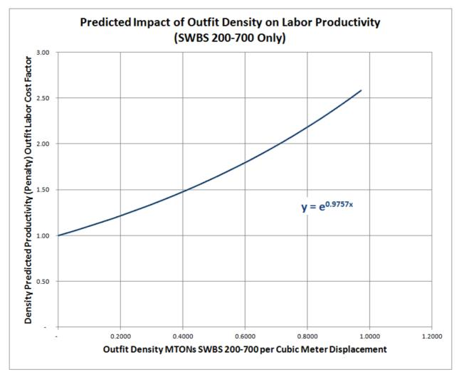
Figure 10 displays relative labor hour productivity as a function of the outfit density. This formula uses large volume, low density ship designs like tankers and bulk carriers for a factor of 1.0. The labor productivity factor then increases exponentially as the density increases.
