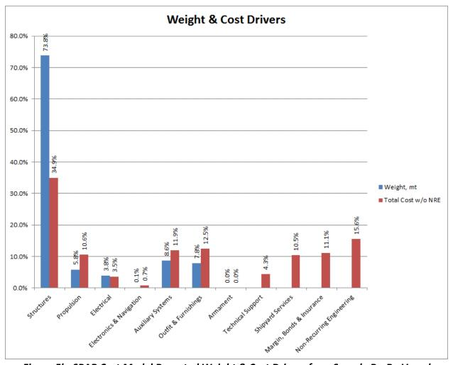
Figure 5b: SPAR Cost Model Reported Weight & Cost Drivers for a Sample Ro-Ro Vessel
