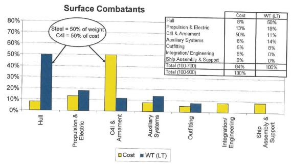
Figure 2: NAVSEA Cost Drivers for Surface Combatants
