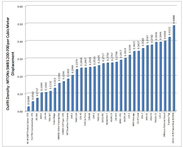
Figure 8 displays density factors as computed for various ships, both commercial and naval:
